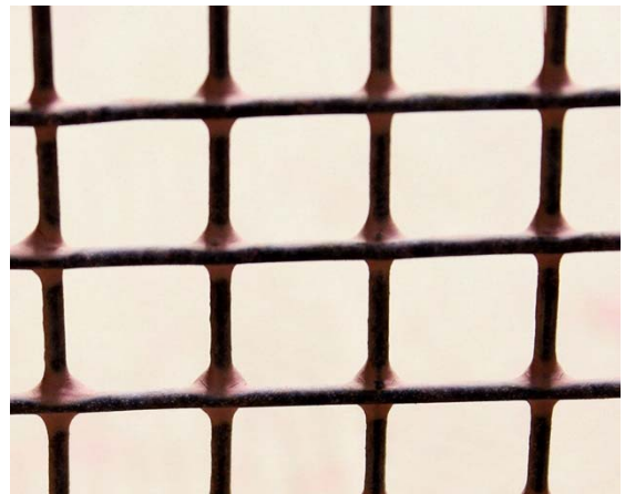
Kiln wash filling corners in screen.
