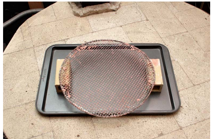
Kiln wash coated screen drying on kiln.
