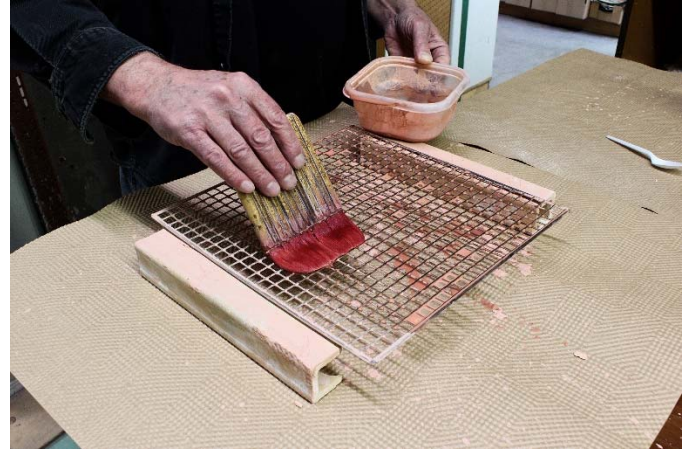
Applying kiln wash to a screen with 1/2 inch grid.
