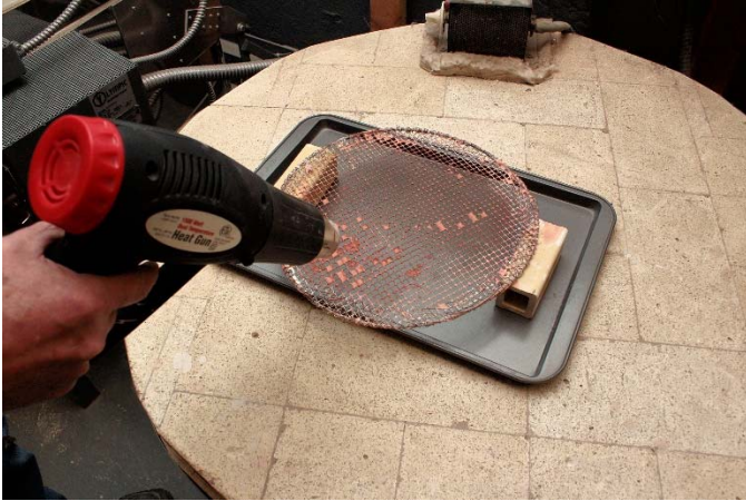
Using a blow dryer to remove film from screen.
