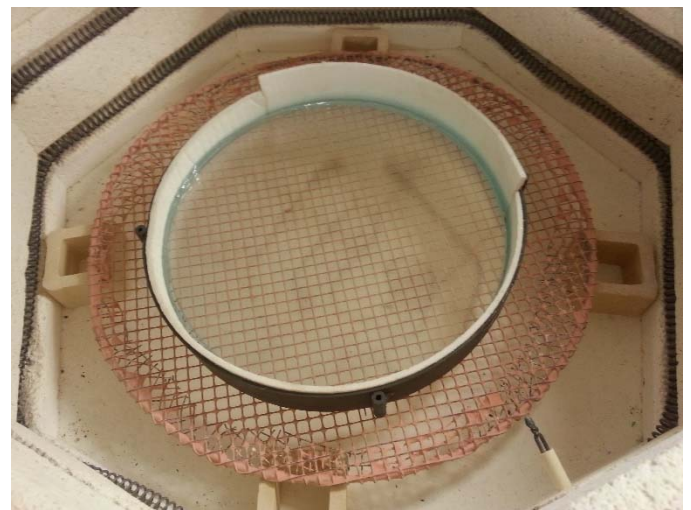
Clear glass in an 8 inch mold on a 12 inch diameter kiln washed screen with 1/4 inch grid spaces.
