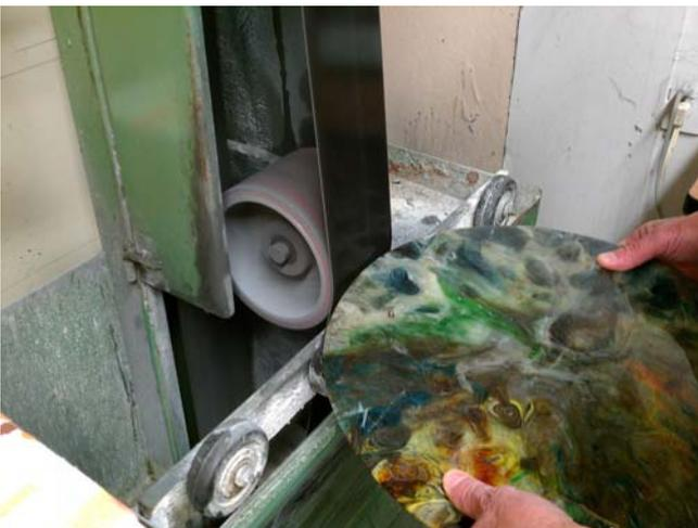
*Edge grinding a screen melt on a Wet Belt Sander*
