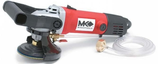
Like an Angle Grinder but with a built-in hose to dispense a steady stream of water while running. These use Velcro-attached 4 inch diameter Diamond Discs in 50, 200, 500, 1000, 2000 and 3000 grit as well as felt for polishing with Cerium Oxide.
