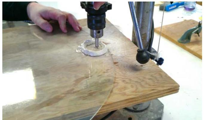
*Drilling a large round of glass using putty to contain a pool of water as coolant.*
