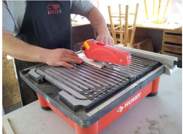
Cutting a glass bar with a Tile Saw
