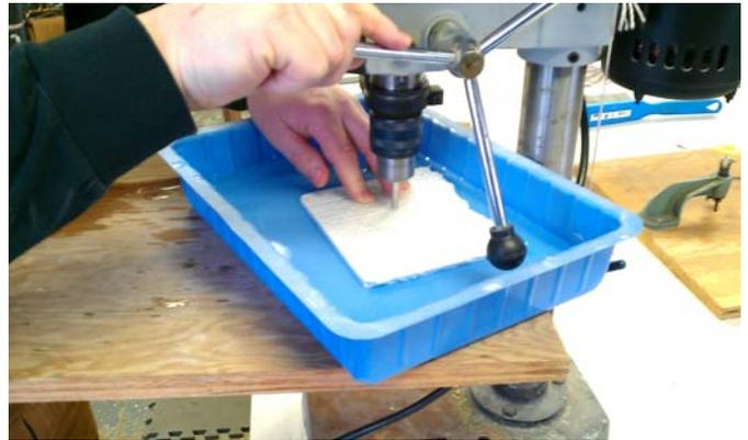
*Drilling a piece of glass in a tray filled with water and a piece of styrofoam beneath the glass*
