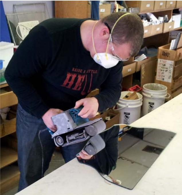
*Edge sanding a mirror with a Silicon Carbide belt*
