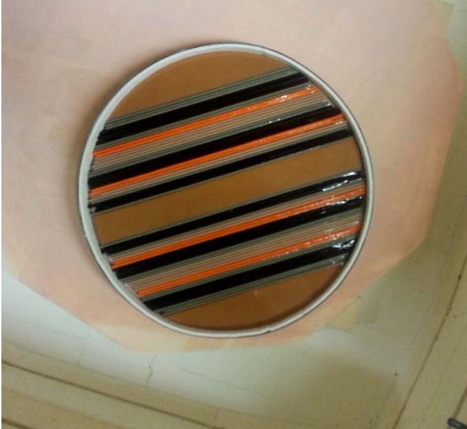
3mm clear glass with 3mm x 6mm strips on top
