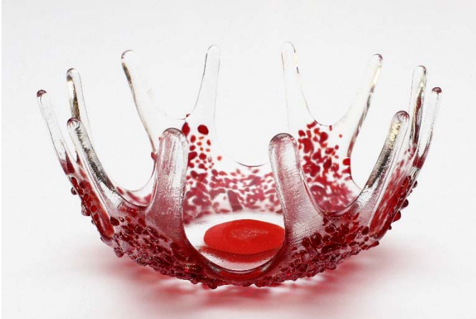
Assembly with red frit tack fused on and draped over a small steel bowl
