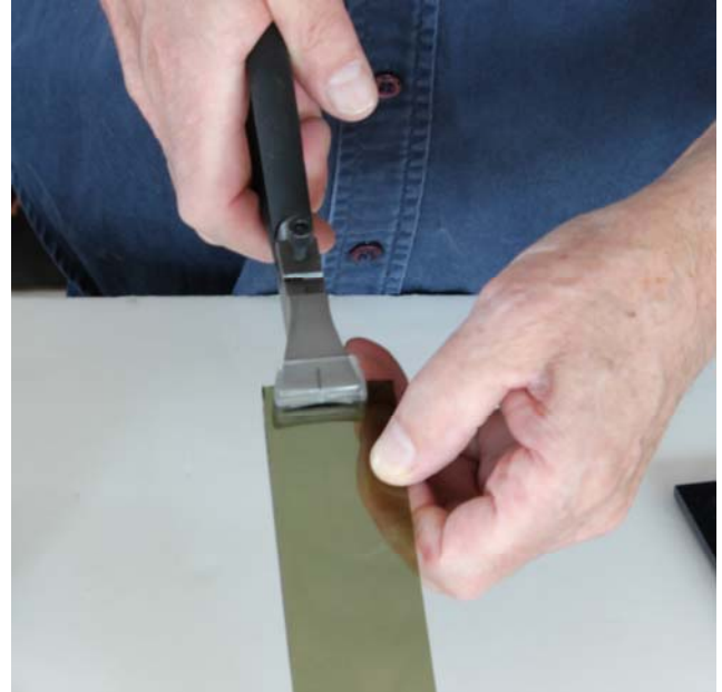
Breaking with Breaking Pliers
