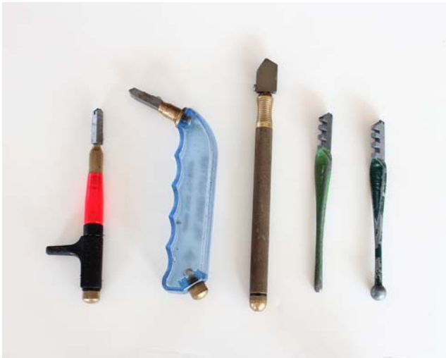
From left to right, “Thomas Grip” cutter, “Toyo” pistol grip cutter, conventional wide tip cutter for thick glass, old style cutter for tapping, old style ball cutter for setting beneath score.
