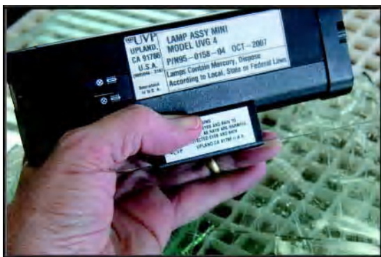
3. To find the tin side of float glass, you will need a shortwave UV light, sometimes called a tin detector or tin scope. The tin side will produce a white glow when the UV light is shone on it at a 45-degree angle.
