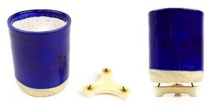
Stilts are ceramic stands with high temperature wire prongs embedded in them. The clay ware stands on the end of the wire prongs. Because the only contact is with the wire prongs, these allow you to fire projects that are even glazed on the bottoms.
