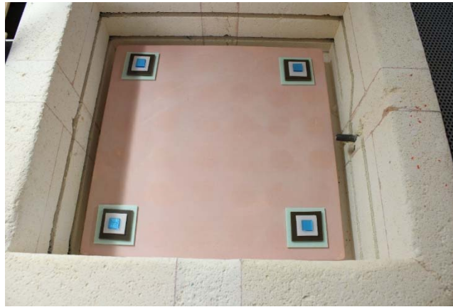
Test stacks at each corner of the kiln ready to fire to test for temperature variance.
