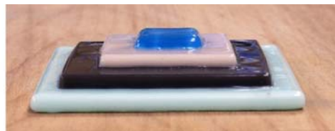
After firing to 1350°F (732°C)
