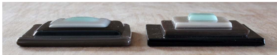
Identical tiles fired in the same kiln at the same firing schedule at different times. The tile on the left was fired with lid elements only. On the right with only side elements
