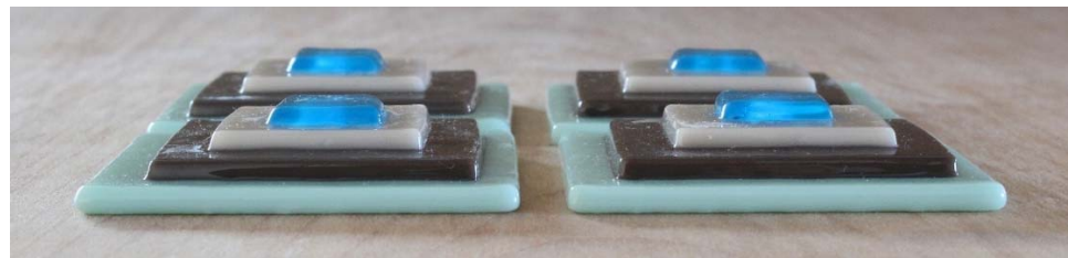
Test stacks after firing to 1350°F (732°C)
