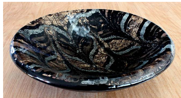
Combed mica project fired in a mold with scraps of clear glass as a cap then slumped into a bowl.
