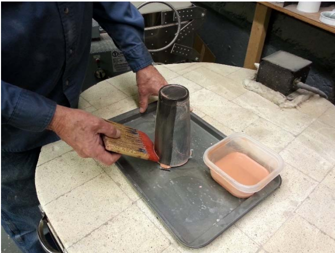
Applying kiln wash onto steel mold on warm kiln
