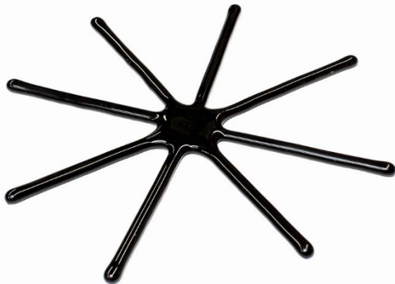
Spider leg assembly after fusing
