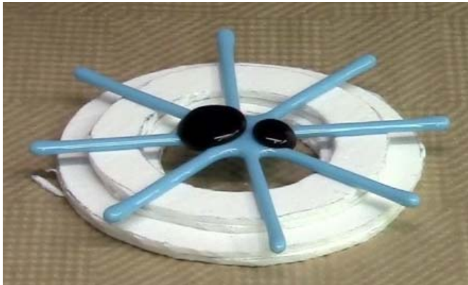
Spider assembly on mold rings ready to slump
