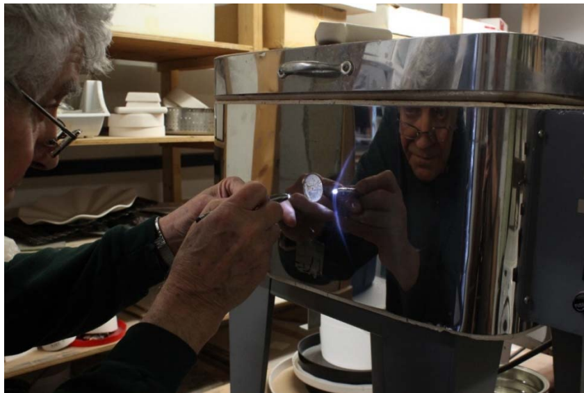
Shining a pen light into the vent plug hole to peep inside.
